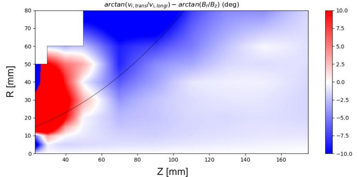
FIGURE : Comparison between ion velocity and magnetic field lines
