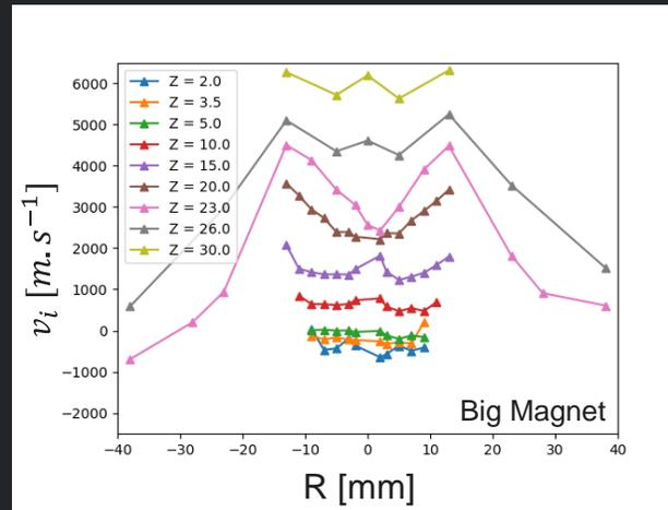
FIGURE : Ion velocity at different axis location in the source of an ECR thruster
